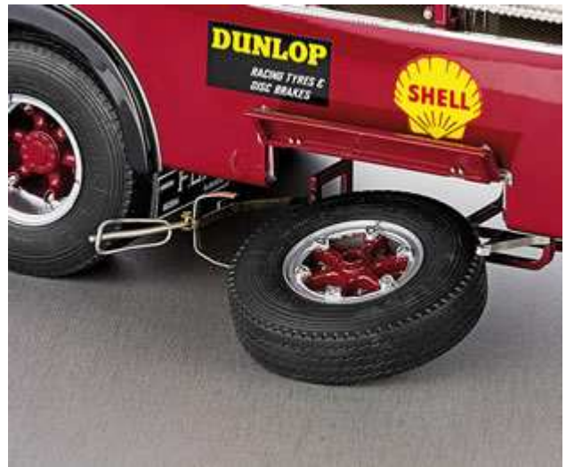
Removable spare wheel and spare-wheel bracket with a functional spring clip-lock
