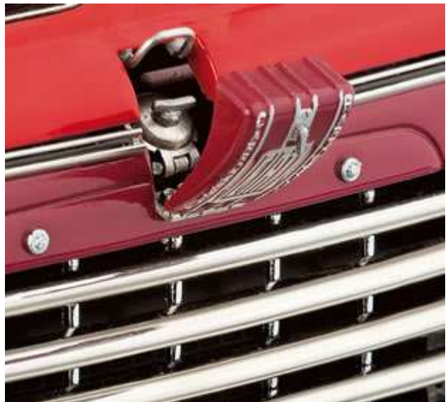
Distinctive radiator grille made with individually-mounted bars of polished metal
