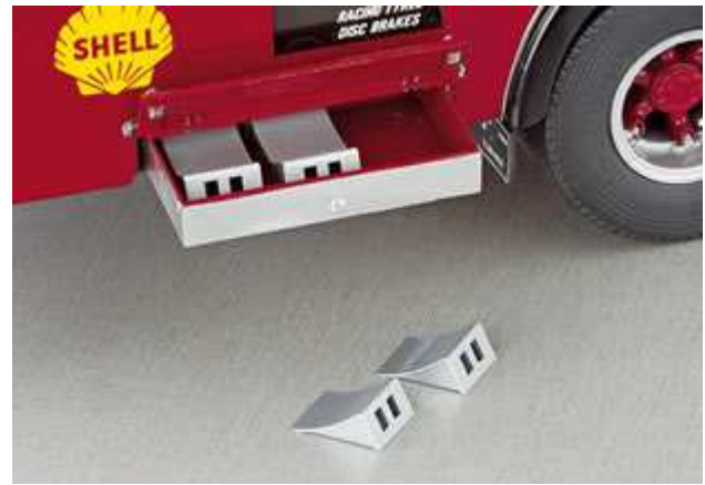
Functional storage drawer. It is designed to stow away the six stop-blocks for holding race cars in place.
