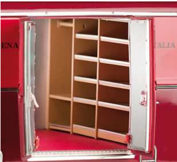
Inspection bay with built-in racks for spare parts
