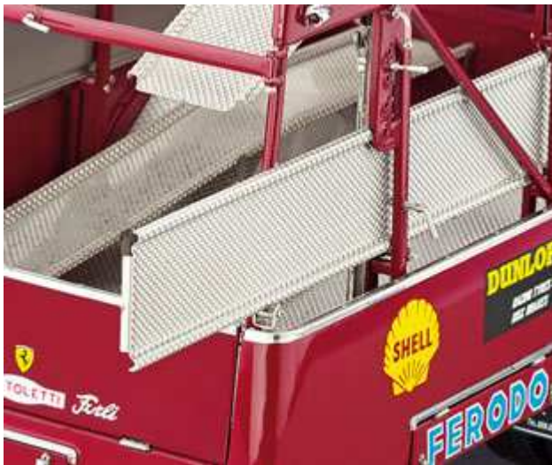
The ramps can be shelved sidewise and held in place with toggle screws.
