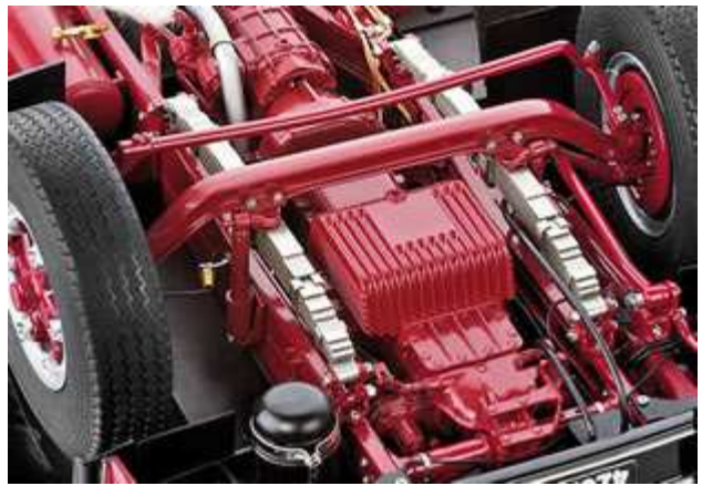
Front axle with metal compound leaf-springs.
