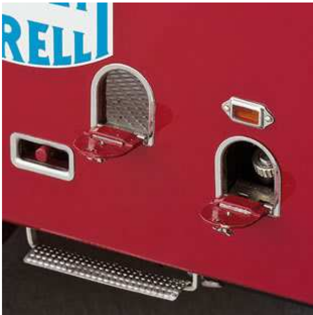
Covers of the fuel filler neck and step can open and close.
