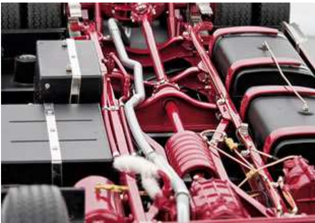
Perfectly-replicated drive chain, which is embedded in a ladder frame of metal.
