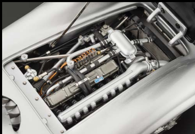
True-to-the-original replication of the 8-cylinder in-line-engine of the W196R, 1954.
