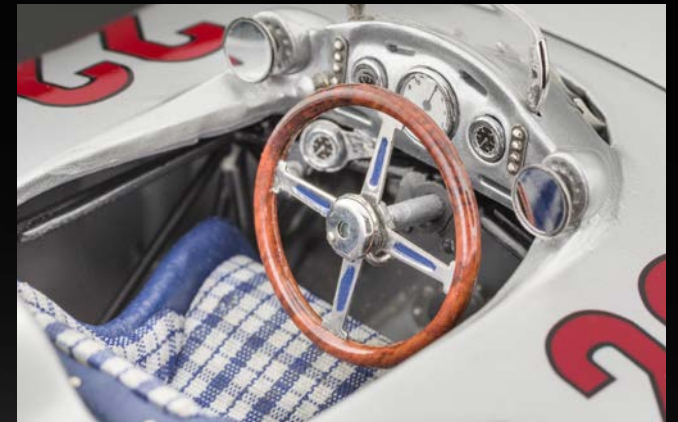
The driver work station is distinctively equipped with a 4-spoke steering wheel and an additional oil temperature gauge below the dashboard.
