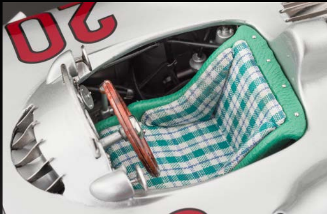
Elaborate seat design, featuring fabric covers and leather trimmings. Beautifully shaped air inlet for cockpit ventilation.
