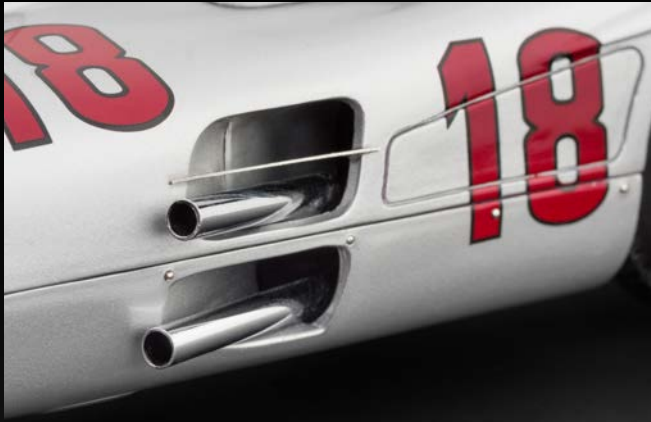
Exhaust pipes come out through two body openings separately. The top opening is mounted with a chromed crossbar.
